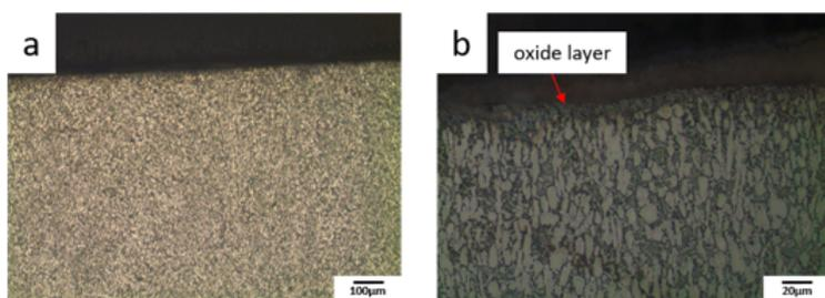
Fig. 4. Cross-sections of microstructures of the sample after heat treatment 10h 450°C a) magnitude x100, b) magnitude x500 (sample 4).
