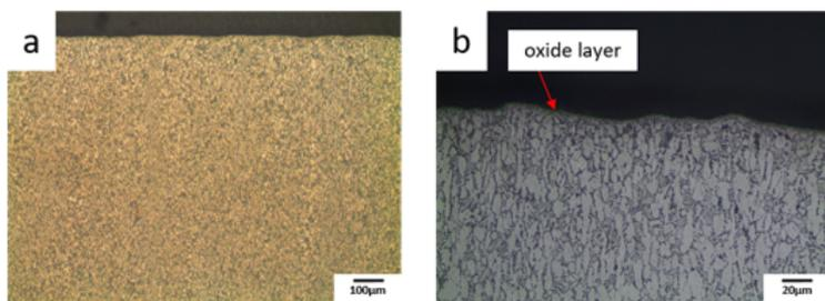
Fig. 2. Cross-sections of microstructures of the sample after heat treatment 5h 350°C a) magnitude x100, b) magnitude x500 (sample 2).
