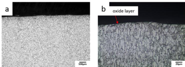
Fig. 5. Cross-sections of microstructures of the sample after heat treatment 1h 550°C a) magnitude x100, b) magnitude x500 (sample 5).
