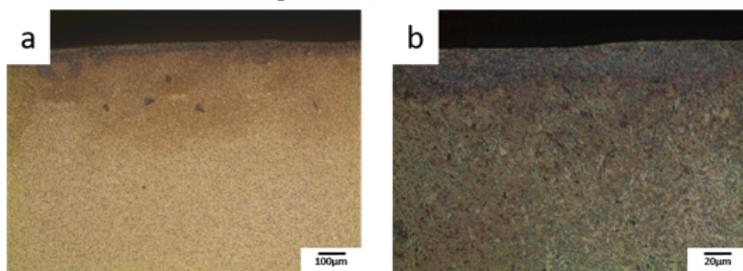
Fig. 1. Cross-sections of microstructures of the sample without mechanical activation of surface a) magnitude x100, b) magnitude x500 (sample 1).
