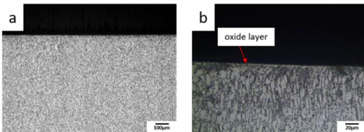
Fig. 7. Cross-sections of microstructures of the sample after heat treatment 5h 650°C a) magnitude x100, b) magnitude x500 (sample 7).
