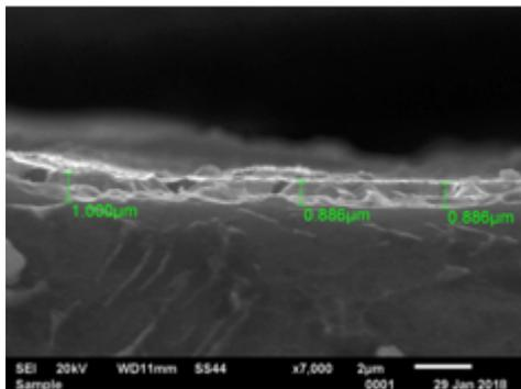
Fig. 8. Way of measuring thickness of the oxide layer - example for the sample after heat treatment 5h 350°C.
