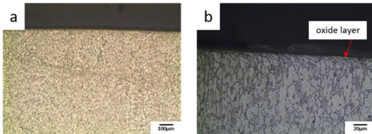
Fig. 6. Cross-sections of microstructures of the sample after heat treatment 10h 550°C a) magnitude x100, b) magnitude x500 (sample 6).
