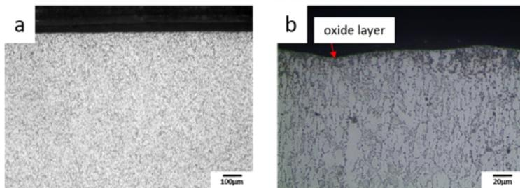
Fig. 3. Cross-sections of microstructures of the sample after heat treatment 1h 450°C a) magnitude x100, b) magnitude x500 (sample 3).
